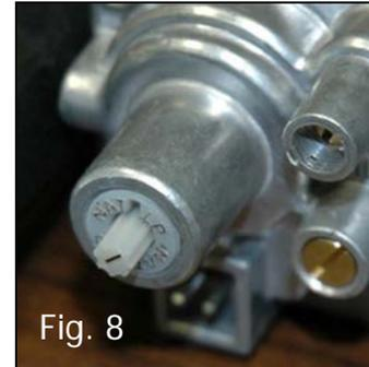
The step motor modulates the flame height at six (6) different levels and automatically calibrates itself to zero when power is first applied via the wiring harness.
